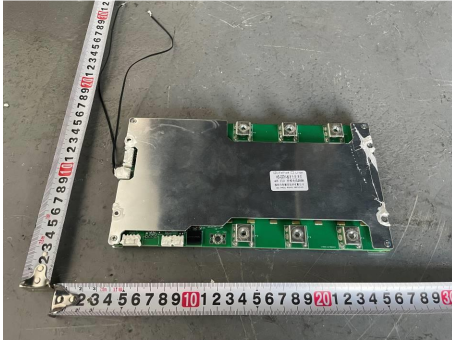
Figure 9 Front view 1 of PCB with BMS
