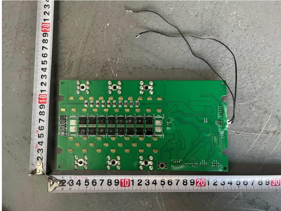
Figure 11 Back view 3 of PCB with BMS
